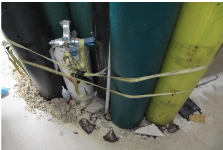
Figure 4: Cluster of ten gas cylinders with shared restraint.
